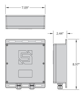
Unit includes two (2) pre-installed 3/8" NPT cable glands for wiring.
