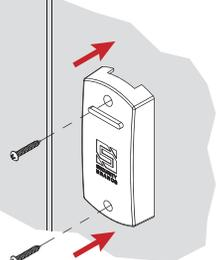
Pre-drill appropriately sized holes if using anchors or if mounting to metal.
