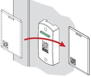
**A5** Hold Reader Base against mounting surface, and use nail to tap two marks.
