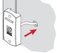
Refer to Wiegand controller instructions for wiring details. If controller only has one LED terminal, connect gray wire (green LED) for standard operation.
