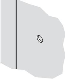
**A3** Feed Reader Base wiring through pass-through hole, and wire reader to Wiegand controller (not included).
