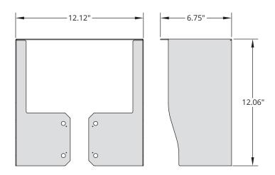
Fits Ascent M8 and secures with existing pedestal-mounting holes.
