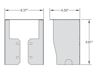
Fits Ascent M3 and secures with existing pedestal-mounting holes.
